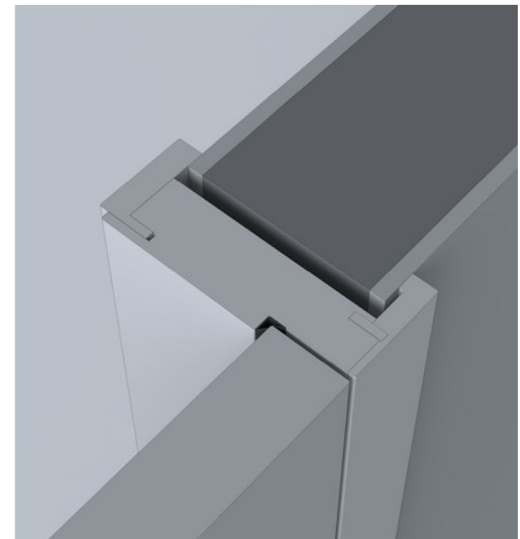
Section of a full casing-covered jamb on one side and an adjustable jamb on the other side, outside flush swing-out.
